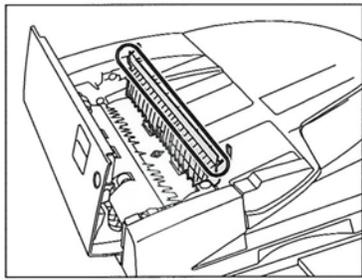
**Step 5** – Clean the transparent plastic part of the inner cover with a cloth dampened with water. Then, wipe the area with a soft, dry cloth.
