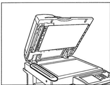
**Step 9** – Clean the feeder scanning area with a cloth dampened with water. Then, wipe the area with a soft, dry cloth.
