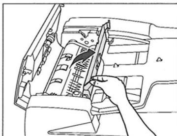
**Step 3** - Open the inner cover, holding it by its front tab.
