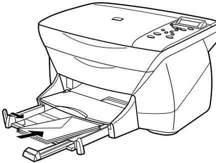
Adjust the left paper guide against the envelopes (be careful not to bend the envelopes). Make sure the envelopes fit within the tray (do not overload it).
