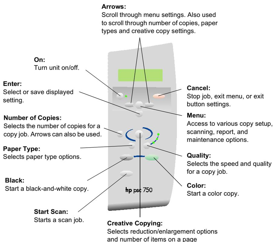
Even if you do not connect your HP PSC to a computer (also called stand-alone use), you can use the front panel to process copy jobs. You can change a wide variety of settings using the front-panel buttons and menu system. Depending on your model, your front panel may look slightly different from the diagram.
